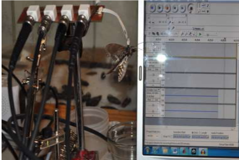
Figure 52: A photograph of the surviving pupae implant moth while the signals are being recorded
